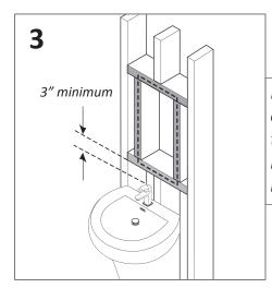
Frame the opening for the cabinet based on the measurement
