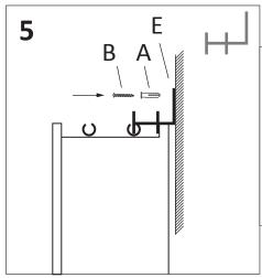
Attach the top mounting bracket to the wall using a screw gun
