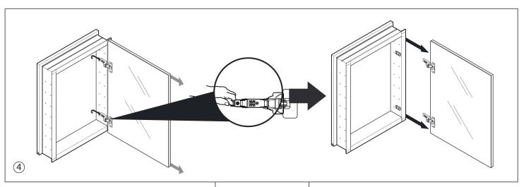
Slide the doors into place by pinching the end of the hinge
