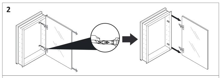
While supporting the door release (the leaver under the hinge arm), slide door off the frame.
