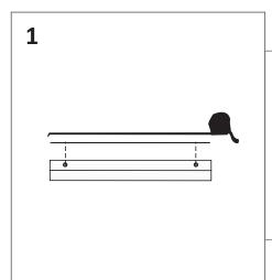
Measure distance between holes for the mounting brackets installation
