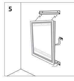
Line up the brackets of the mirror with wall brackets and slide the mirror down
