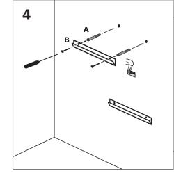
Insert anchors into predrilled holes and fix the mounting brackets to the wall
