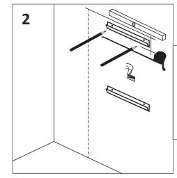
Mark hole positions on the wall ready for drilling
